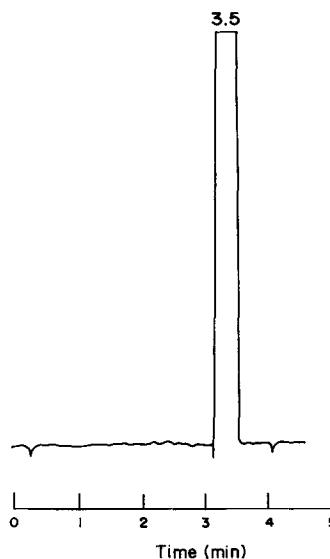
Figure 3 Ratio chromatogram of a liquid sample; the wavelengths used were 278 and 270 nm.
